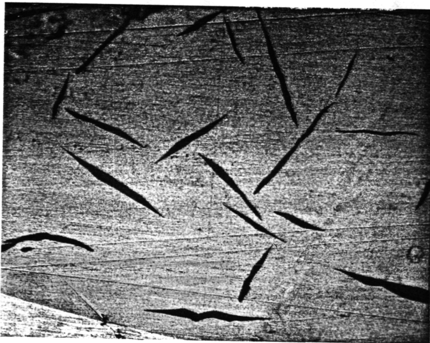
Figure 19. Eutectic solidified at 2.7 mm/hr, 150X.
